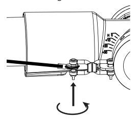
Lock both swivel pins in place by threading locking (mousing) wire through the hole in the head of the swivel pin and wrapping it around one of the arms of the swivel! Make sure both swivel pins are locked to the swivel with mousing wire!
