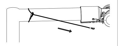
Pass the swivel pin through smaller thimble and tighten!
