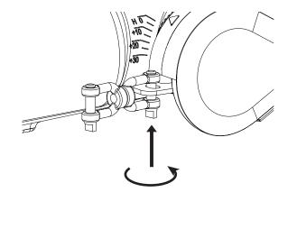
Release and remove other pin from swivel!
