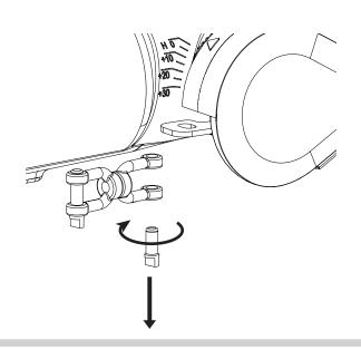
Install swivel to lantern and tighten pin!
